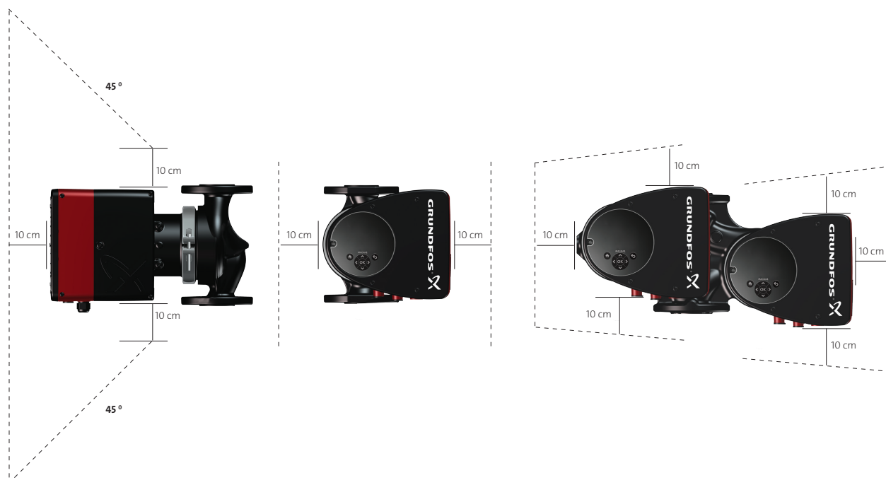
Minimum clearance around Twin-head pump
